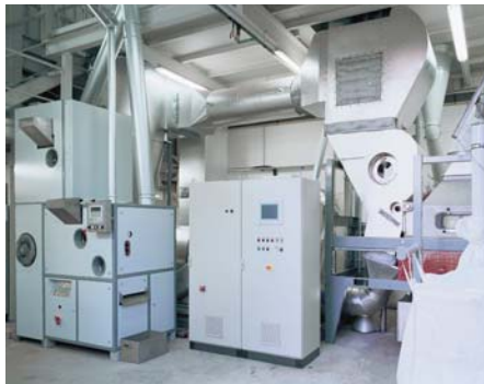
NEUHAUS NEOTEC pilot plant at Ganderkesee near Bremen for coffee processing, fluidized bed agglomeration, and roller mills.
