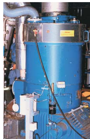
Pelleting press for pelleting of sewage sludge in Nuremberg.
