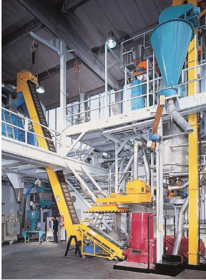
KAHL pilot plant with proportioning unit, continuous mixer, hydrothermal reactor, annular gap expander, extruder OEE, flat die pelleting press, belt drier/cooler, Rotospray, crumbler.
